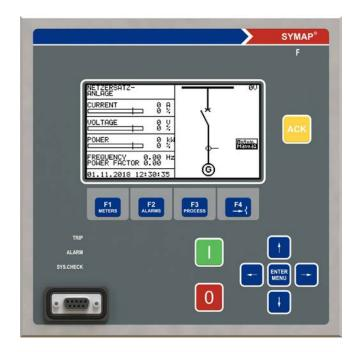
all active alarms, event log and blockings. »Process« shows all process data such as the synchronization display, motor thermal indication and a counter of breaker operations. Under »Breaker Control«, up to five breakers can be accessed and controlled.
